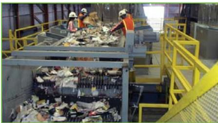
Materials are separated with the work of machines and people at the Material Recovery Facility (MRF).
