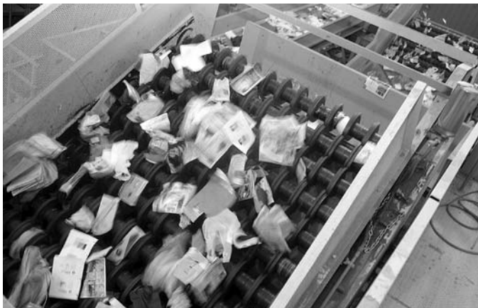
Above, BHS's News Sorter system. Below, a vacuum system designed for removing fiber from a conveyor belt directly to a baler.
