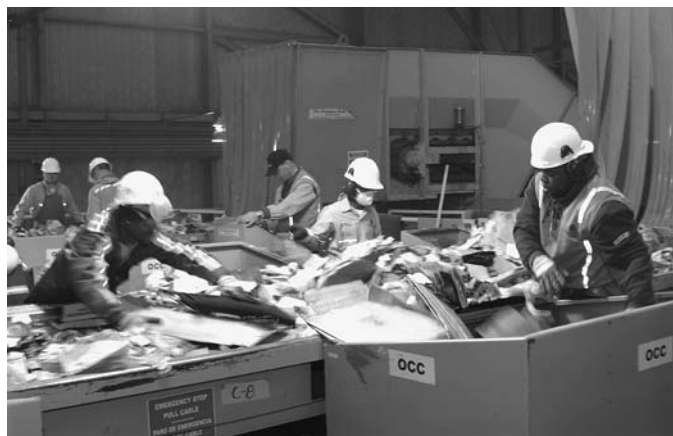
Above, workers sort Old Corrugated Containers for baling. Below, a baler producing a serpentine-like bale.
