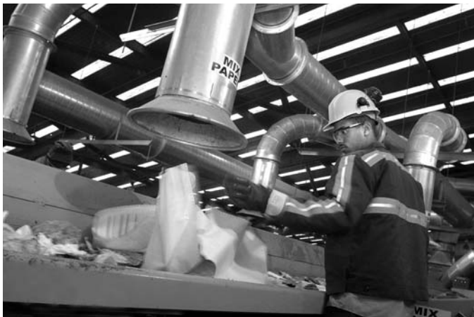
Above, BHS's News Sorter system. Below, a vacuum system designed for removing fiber from a conveyor belt directly to a baler.
